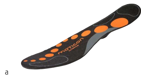
Fig 3a–b Appearance and sensor distribution on the OpenGo.
